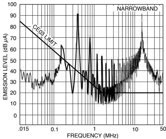
Two MGH2805S converters at full load, no filtering.
