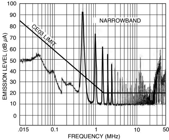
Two MGA2805S converters at full load, no filtering.
