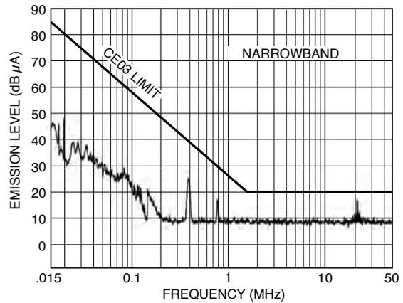
Two MGH2805S converters at full load with FMGA-461 filtering.
