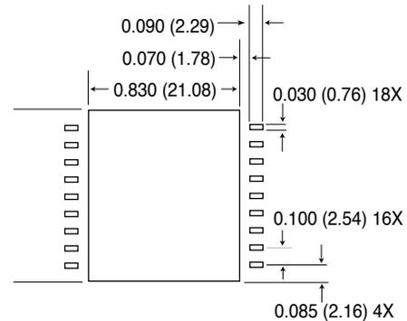
The triangle (ESD) marking on the cover indicates pin one. Cover marking is oriented with pin one at the upper right corner. The straight lead configuration does not require a "case designator" in the model number. ex. FMGA-461
