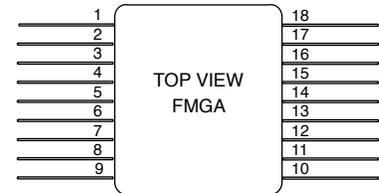
Differently colored glass bead around pin one or dimple in header (bottom or side of case) indicates pin one. Cover marking is oriented with pin one at the upper right corner.
