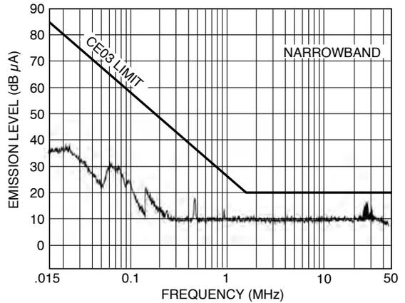
Two MGA2805S converters at full load with FMGA-461 filtering.
